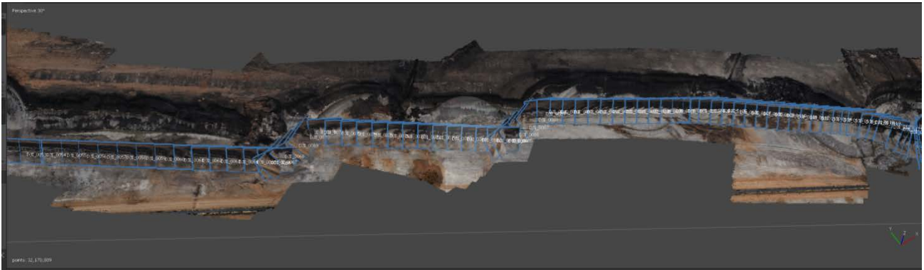
Figure 7. Dense cloud and images captured by P4P in Agisoft Photoscan Pro® [11]
