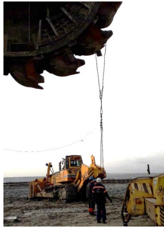
Figure 76 Attachment of the auxiliary machine to the bucket
