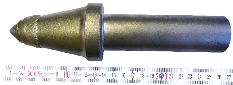
Figure 1. The point attack pick BETEK BSR283 adapted for the hammering device.
