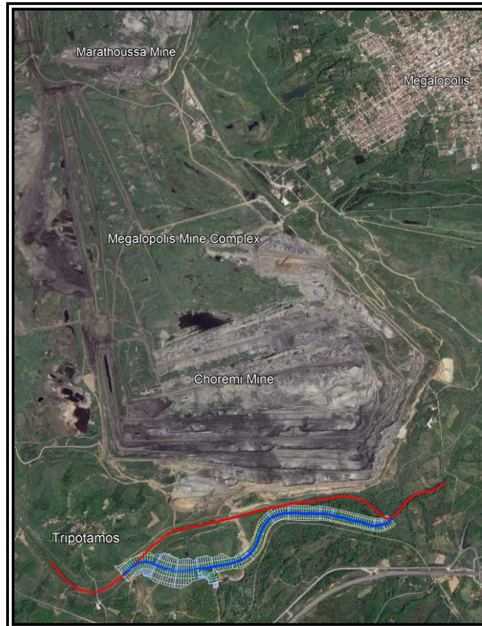
Figure 146. Layout of the south-most part of the Megalopolis Mine Complex. The red line designates the existing Alfeios channel. The blue line to the south corresponds to the axis of the sectional diversion project.
