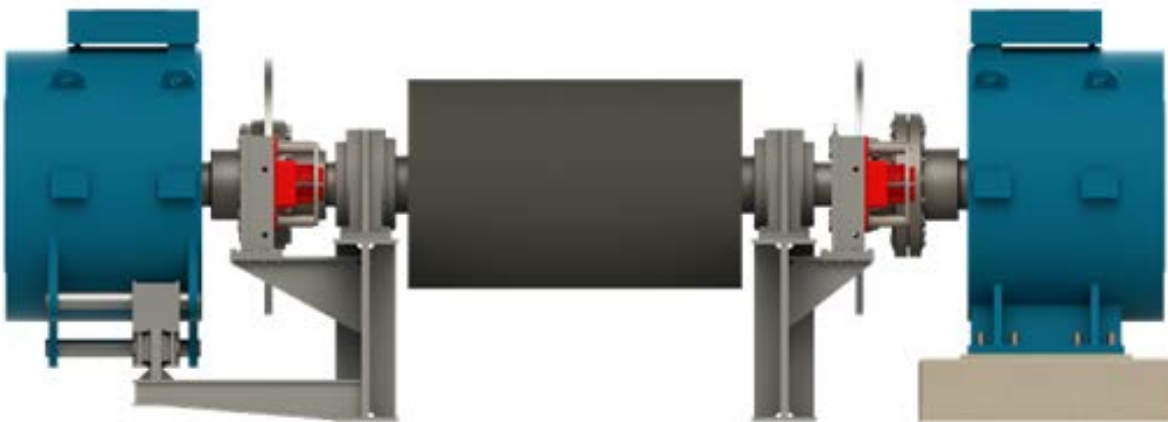
Figure 4. Foot-mounted (right) and shaft-mounted (left). The motor mounted to and suspended by the pulley shaft has favourable characteristics, such as quick installation or swap-out. However, the foot-mounted version is the easiest to design and dimension, especially as the motor weight has no influence on the dimensioning of the pulley shaft. The choice depends on customer preference.
