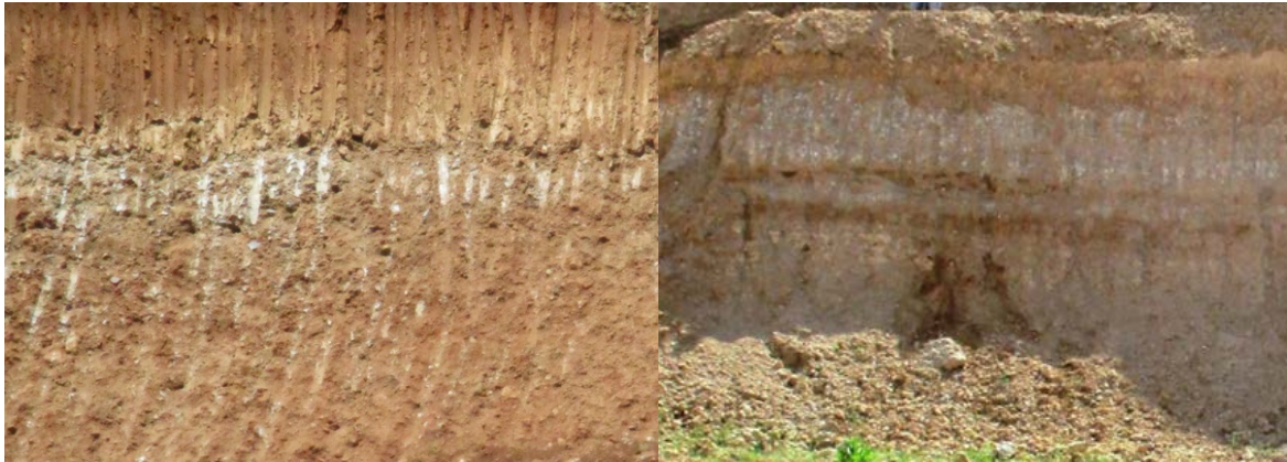
Figure 1. Typical hard rock formations (consolidated conglomerates) occurring during overburden removal in South Field mine in Ptolemais, Greece. (Left): Thin hard rock layers within clay beds which can be difficultly excavated by BWE. (Right): Thick hard rock formations requiring blasting and removal by shovels and dumpers (Provided by PPC).
