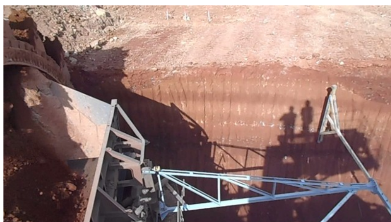
Figure 12. Photograph of the mine face during the excavation. Thin hard and semi hard layers are interbedded within the reddish clays.
