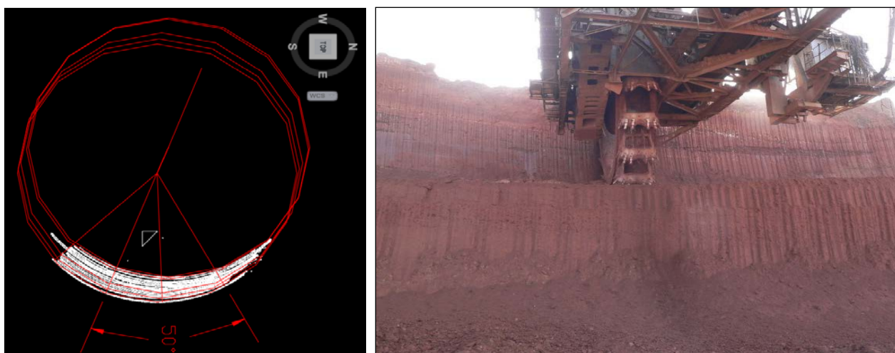
Figure 8. (Left) Trajectories of the BW, slewing angles and angular location of buried boulders at 50° from the advance direction axis. (Right) Mine face at the start of the field test. Within the reddish clay formation thin hard and semi hard layers are interbedded.
