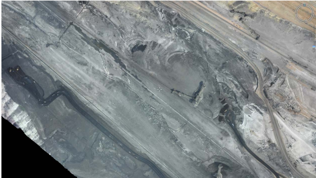
Figure 8. Water intrusion from a channel in a fault zone
