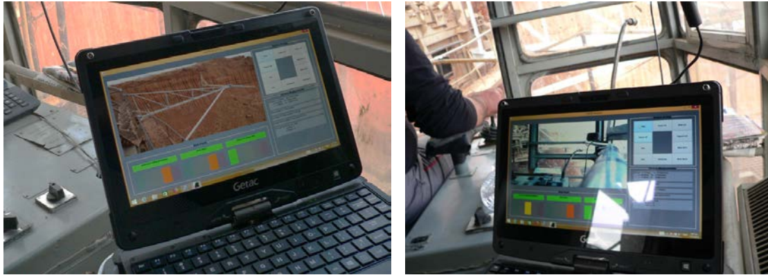
Figure 10. Visualization of the results of the real time inspection system on laptop screen in the operator cabin. In the left photo the camera was installed outside the cabin focusing on the excavation area. In the right photo camera was installed inside the cabin providing a more general view. In both photos the probability of hard rock occurrence, the BWE effort and the risk of collision are displayed using a five level color scale.
